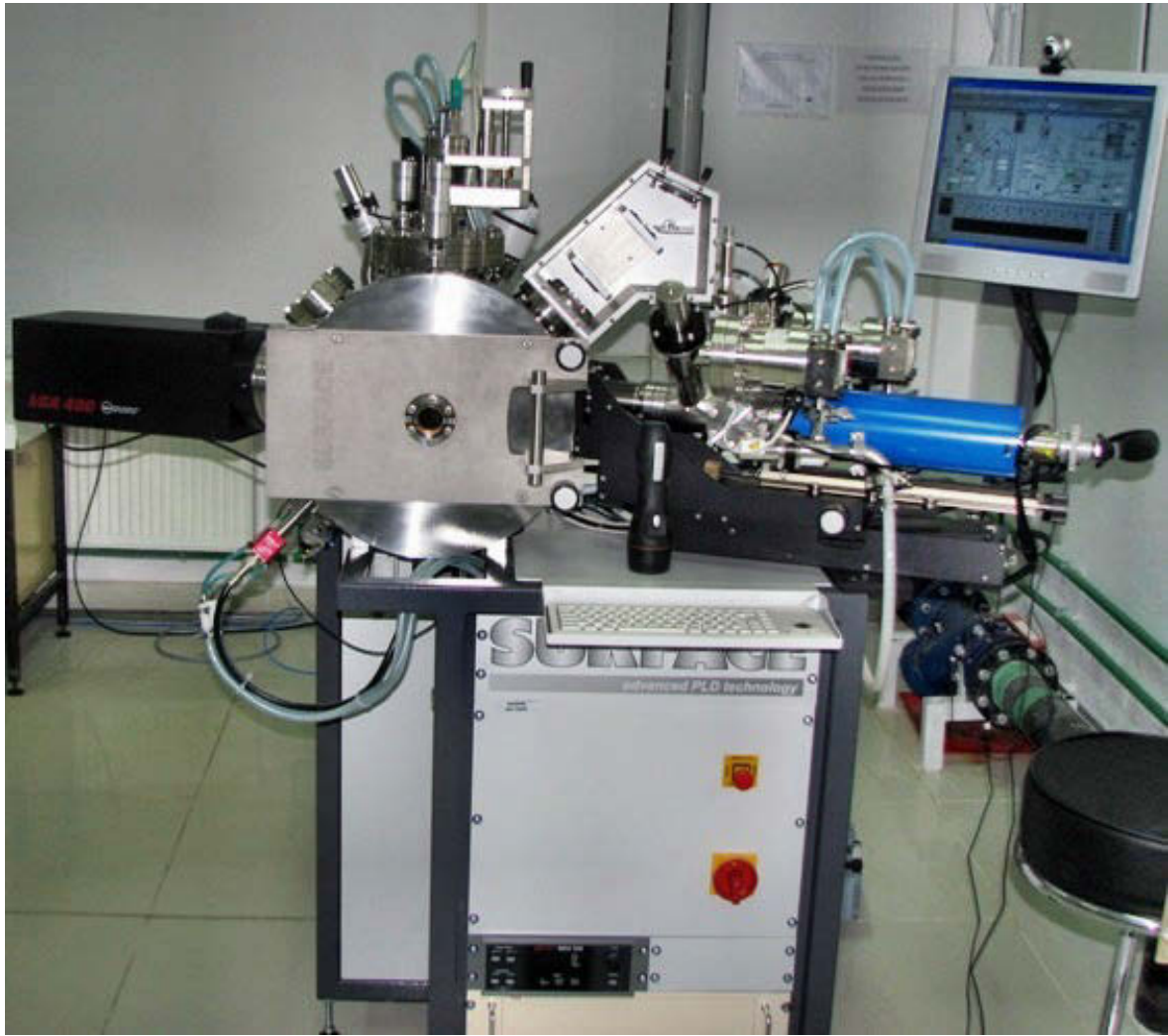
Figure 2.4: The PLD experimental set-up used for the growth of PZT thin layers.
